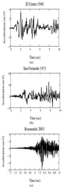
Fig. 8.Accelerograms : (a) El centro PGA =3.41 m/ s $^2$  , (b) San Fernando , (c) PGA =12.02 m/ s $^2$ , Boumerdes PGA =5.77 m/ s $^2$
