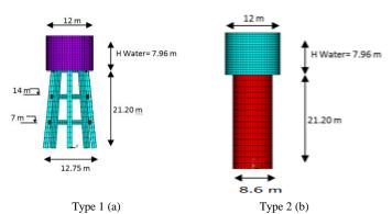
Fig. 2. Elevated tank geometries
