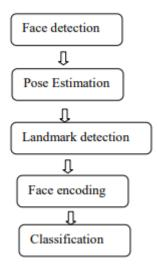
Figure 5 Flowchart depicting face recognition pipeline
