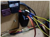
Figure 3 Servo motor for simulating door lock 3.2.4 Notification service
