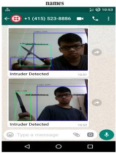
Figure 11 Notification alerts received via Twilio API 4.1.3 Sensor Module
