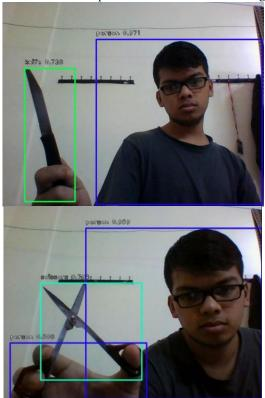
Figure 10 Weapons detected and labelled with their
