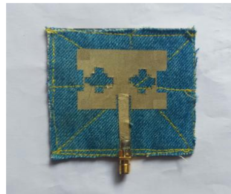
Fig. 6 Demonstrated modified geometry of revised wearable fully textile antenna.
