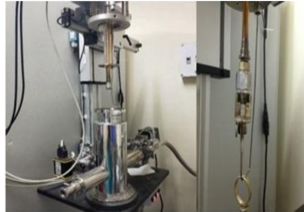
Fig.1 Measurement of fabric properties on dielectric Broadband spectrometer
