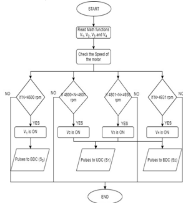
Fig. 7. Flow chart for MFB Controller implementation.
