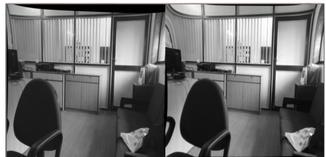
Figure 5: Rectified stereo image captured by the system
