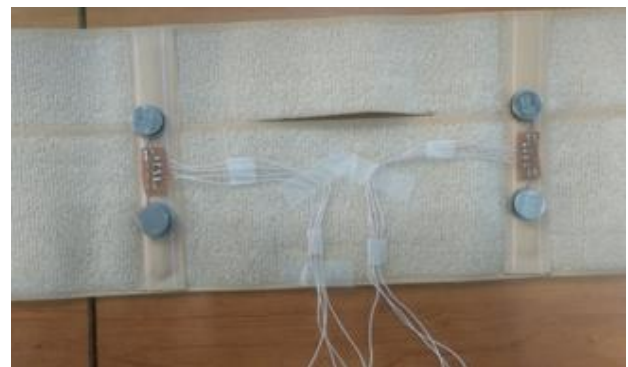
Figure 2: Arrangement of vibrators on orthopaedic belt
