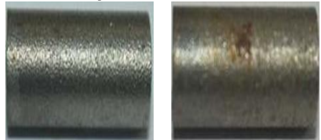
Figure 1(a). Laser sintered Inconel 718 component before corrosion
