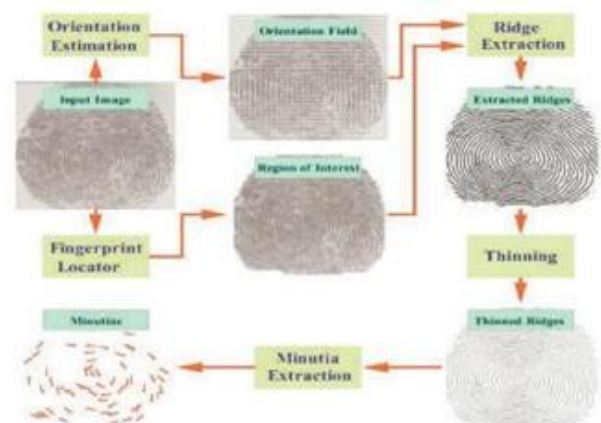
Figure 4: Schematic representation of fingerprint system [10]
