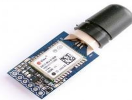
Figure 16: u-blox NEO-6Q GPS MODULE
