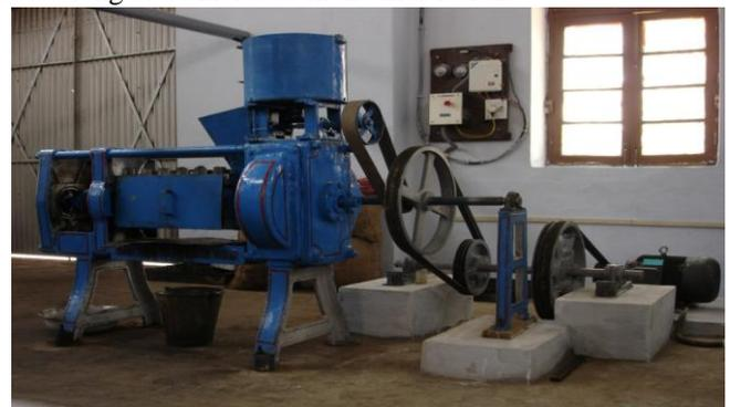
**Fig. 3: Expeller machine for the extraction**
