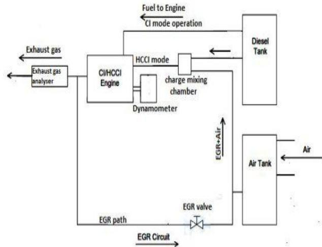
Fig. 1. Layout of engine block schematic
