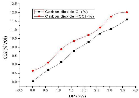
**Fig. 13. CO<sub>2</sub> Vs BP at CI and HCCI**
