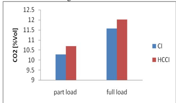
**Fig. 14. CO<sub>2</sub> Vs BP at CI and HCCI part and full load condition**
