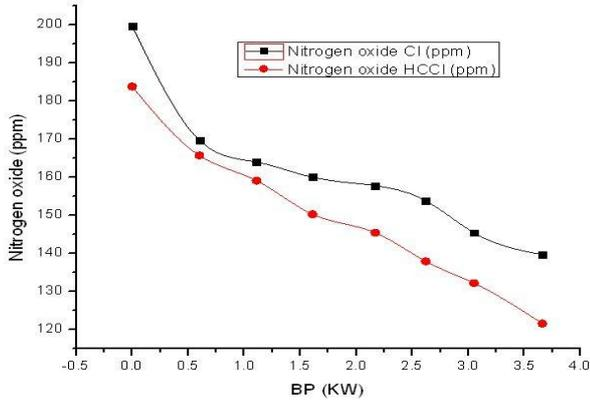
**Fig. 9. Nitrogen oxide Vs BP at CI & HCCI**
