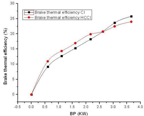
Fig. 3. Brake thermal efficiency Vs BP at CI and HCCI operations
