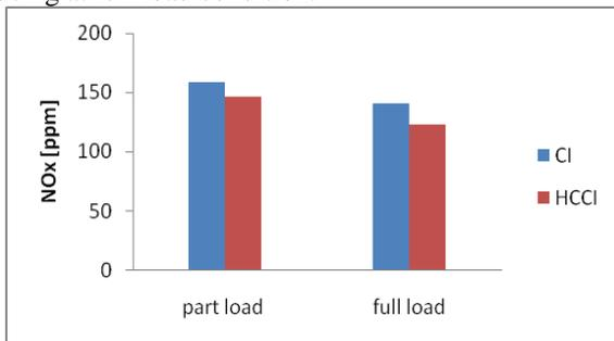
**Fig. 10. Nitrogen oxide Vs BP at CI & HCCI part and full load condition**
