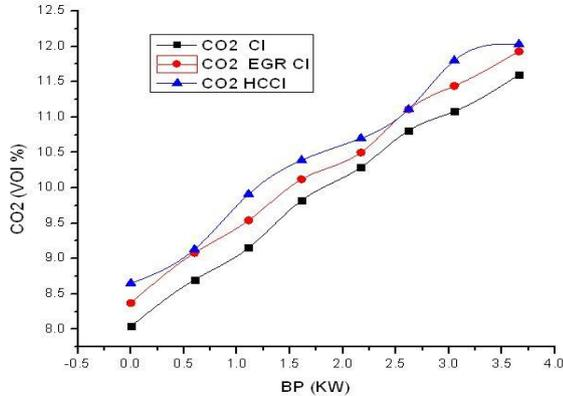
Fig. 19. CO<sub>2</sub> Vs BP at CI, EGR CI and HCCI
