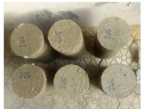
Fig. 4. Demolded specimens (Example concrete 50% Typha)
