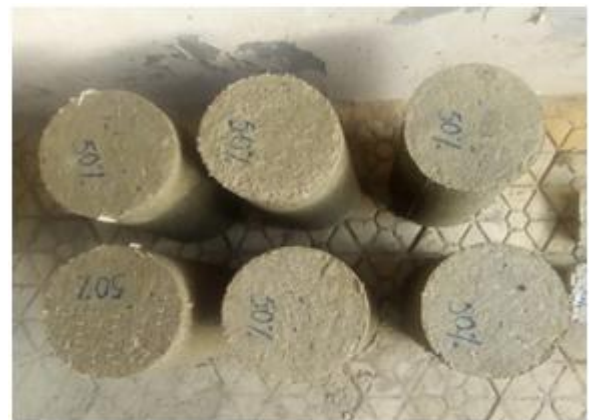
Fig. 4. Demolded specimens (Example concrete 50% Typha)
