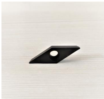
Fig.2. Prepared turning insert
