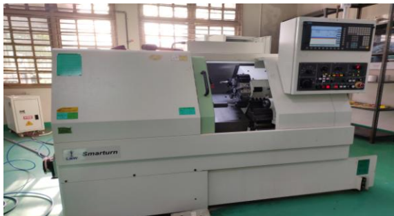
Fig.1. CNC Turning machine used for experimentation
