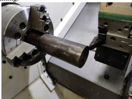
Fig.3 Cutting tool insert fixed in the tool holder
