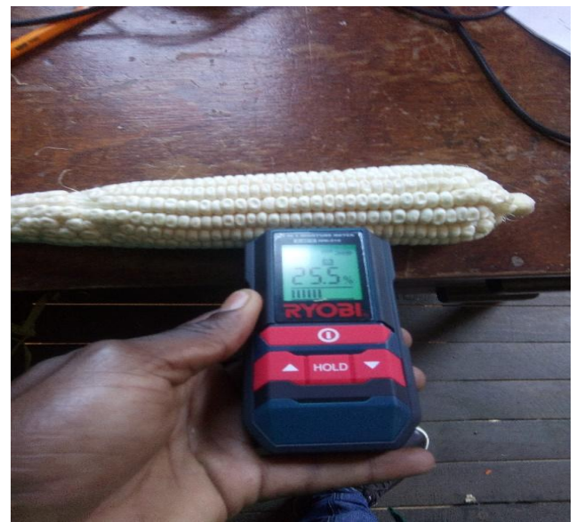
Fig. 3. Sample maize cobs (left) and moisture meter (right) measuring the moisture content of one of the dehusked maize cobs
