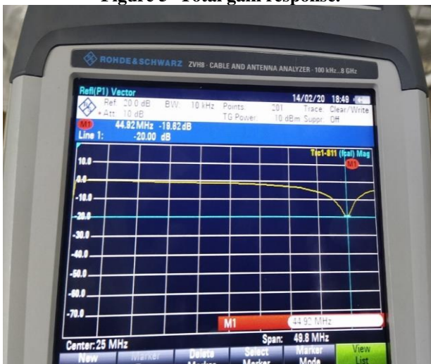
Figure 6- Antenna response (Tuned at 44.92 MHz)
