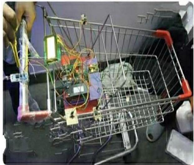
Fig.2 Prototype of smart trolley system
