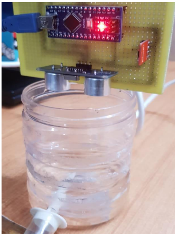
[Fig. Placement and Working of Physical Transmitter Circuit of IoT Based Smart Bottle Sensor]
