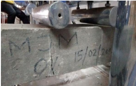
Fig.2 Concrete Beam under Two-point Flexural Load
