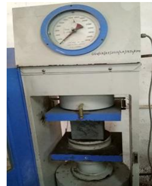
Fig. 1. Concrete cube under compression.
