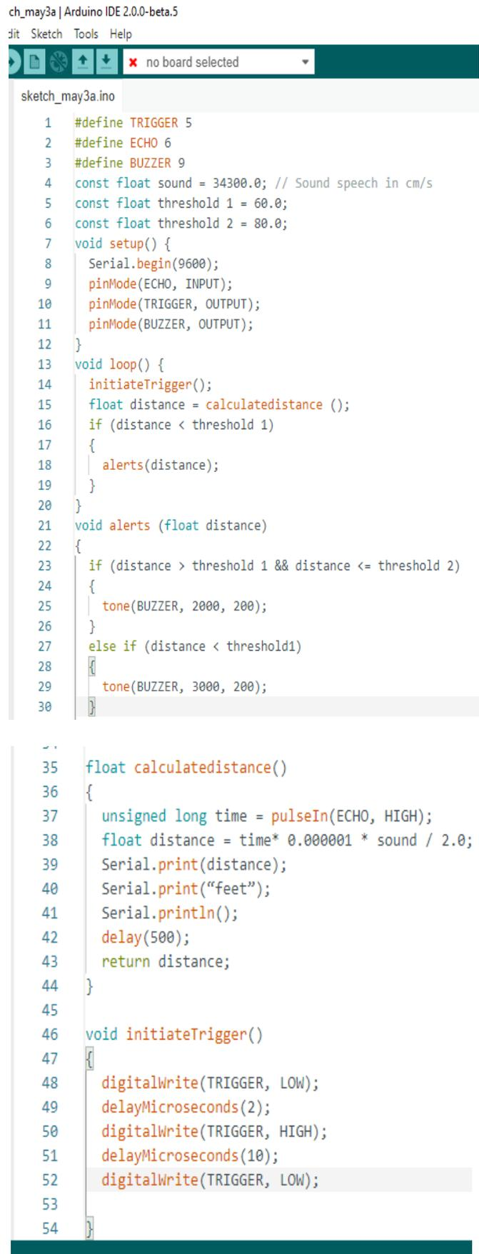
**Figure 4: Coding for Proposed Model**
