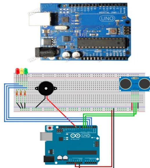
**Figure 2: Arduino UNO Board and Connectivity of UNO Board, Ultrasonic sensor & Buzzer**
