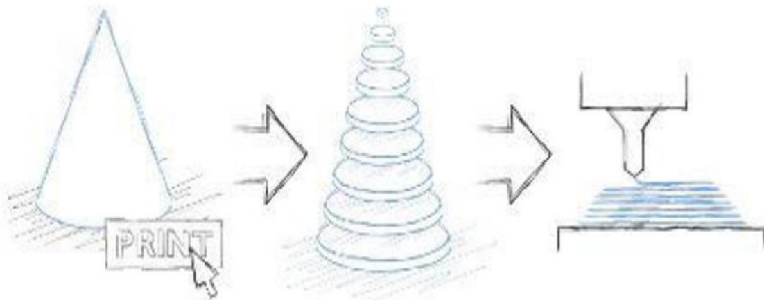
Figure 1 Stages of 3D concrete printing
