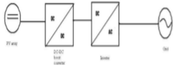
**Fig. 3. Block Diagram of Transformer less Inverter with DC-DC Boost Converter**
