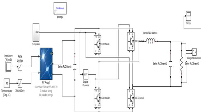
Fig. 4. SIMULINK Model of Transformer Less Self Commutated PV Inverter
