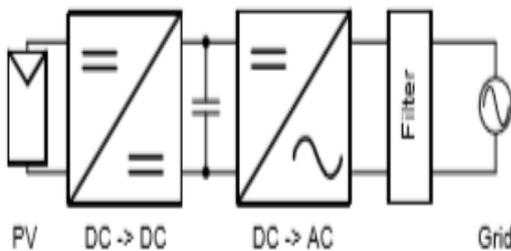
**Fig. 2. Two stage grid connected PV inverters including Voltage Boost**
