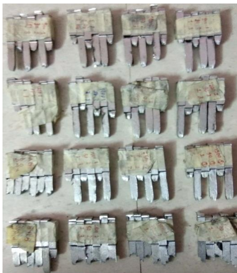
(II) tensile specimen after fracture
