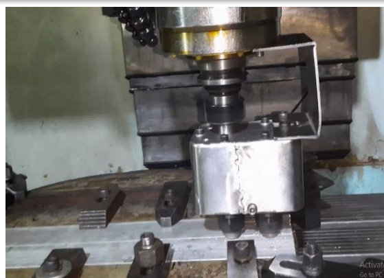
Figure 2 (I) Jyoti VMC 850 set up (II) Twin tool setup
