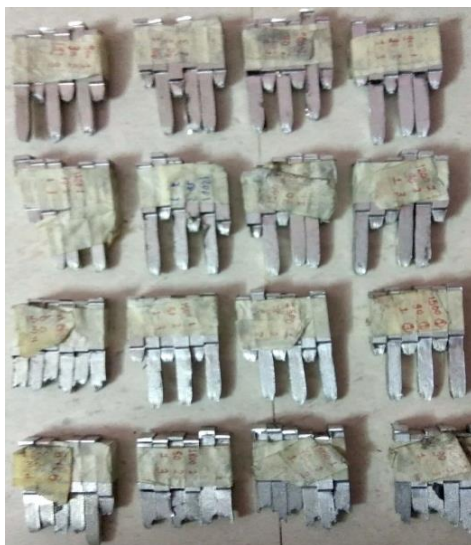
(II) tensile specimen after fracture
