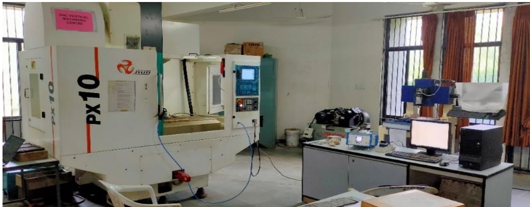
Fig. 4 Vertical milling Centre with KISTLER dynamometer
