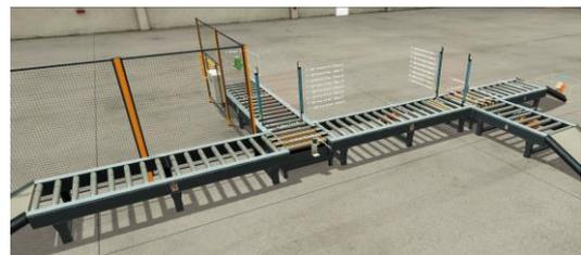
Fig. 5. Production line controlled by Siemens S7-1214DC controller, visualization done in Factory I/O
