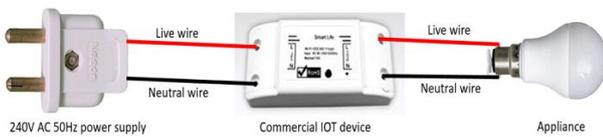
**Fig. 2. Circuit diagram of commercial IOT device**
