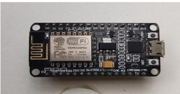
**Fig. 3. NODEMCU AMICA V1.0 Development Board**
