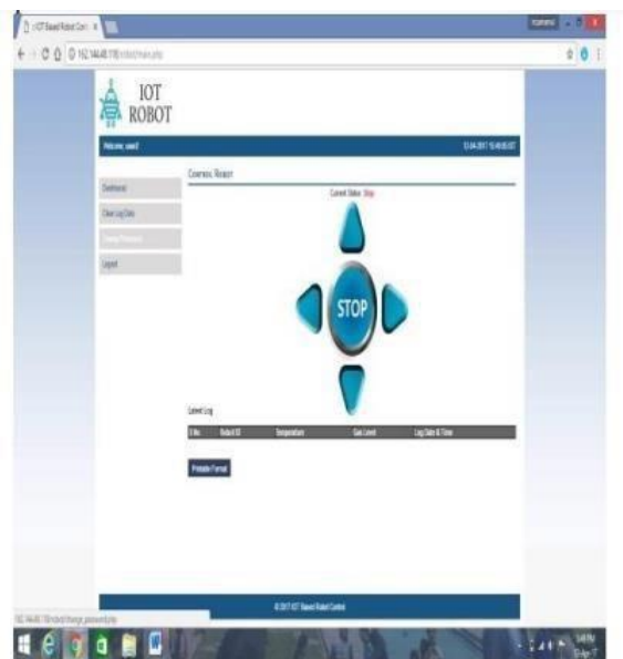
Fig. 6 Robot controller and IoT server
