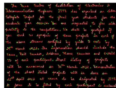
[Fig.4: Boundary Detection in Binary Image. Red trace represents the Boundaries, and Green Star Represent the Starting of the Boundary Pixel]
