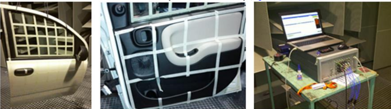
Fig. 10. Trimmed Door Modal Testing Set-up [11]
