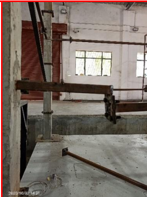
Fig. 10(c) Steel-to-Steel Joint Failure at 2.0g
