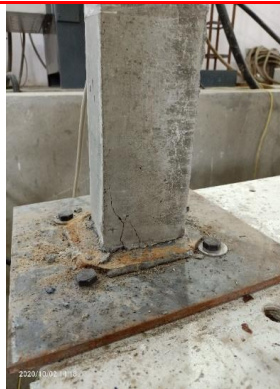
Fig. 10(a) Precast RCC column, Crack from Base at 0.6g
