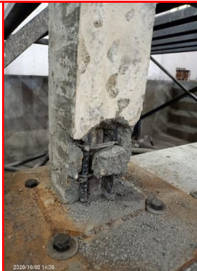
Fig. 10(b) Precast RCC column, Crack from Base at 2.0g
