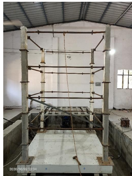
Fig. 4(b) 1/4th PSRC Scaled Model mounted on Shake Table
