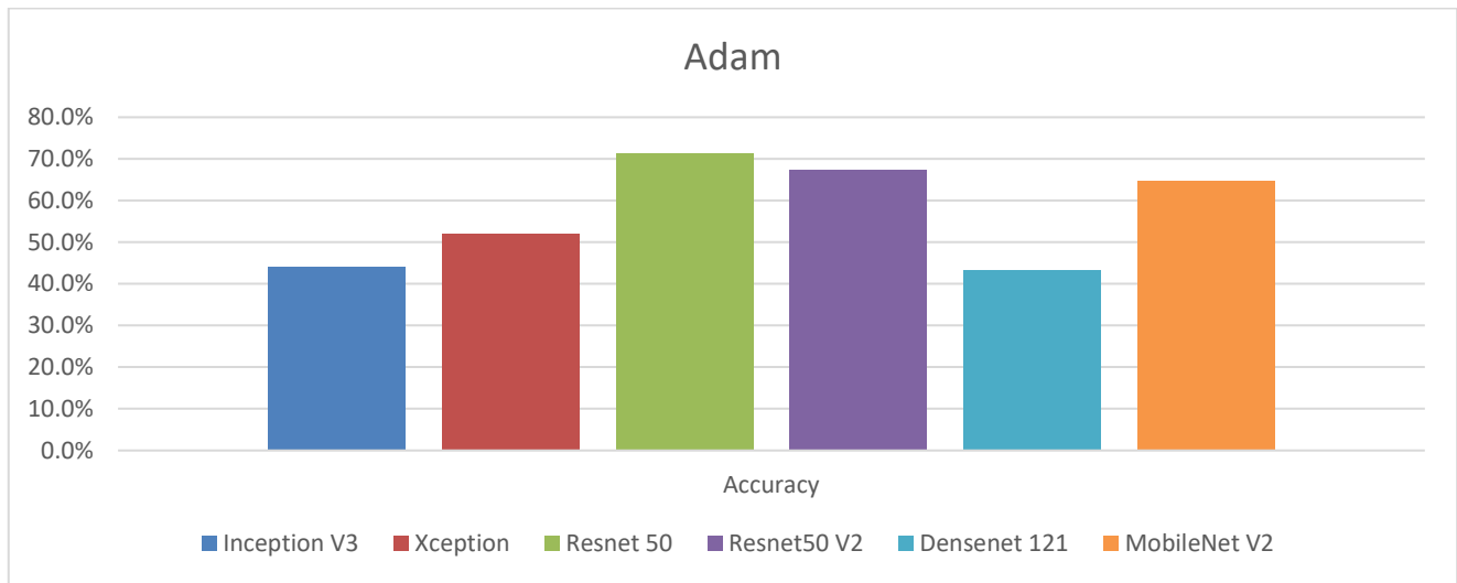
Figure 25. Comparison of accuracy for the Adam optimiser with various models using the Sigmoid activation function.
