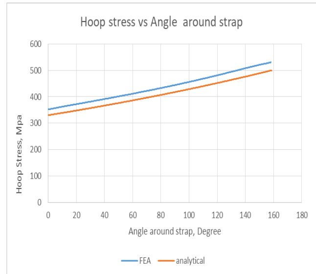
Figure. 7. Comparison of Hoop Stress from FEA and Analytical Results
