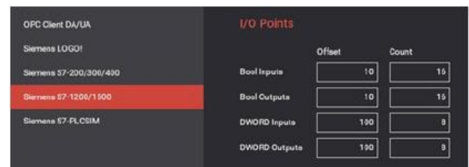
Fig. 3: Configuration in Factory I/O Software of PLC S7-1214 DC/DC/DC
