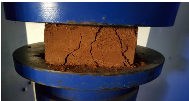
Figure 2. 9: Crushing Strength or Compressive Strength Test on Bricks
