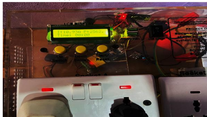
[Fig.12: Picture of the Implemented System for Current of 10.93A]
