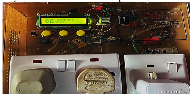
[Fig.14: Picture of the Implemented System in an Overloaded Condition]
