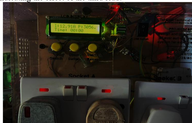
[Fig.13: Picture of the Implemented System for Current of 12.91A]
