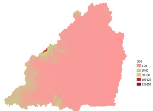
Fig. 3: Filled DEM of Study Area Generated from QGIS
