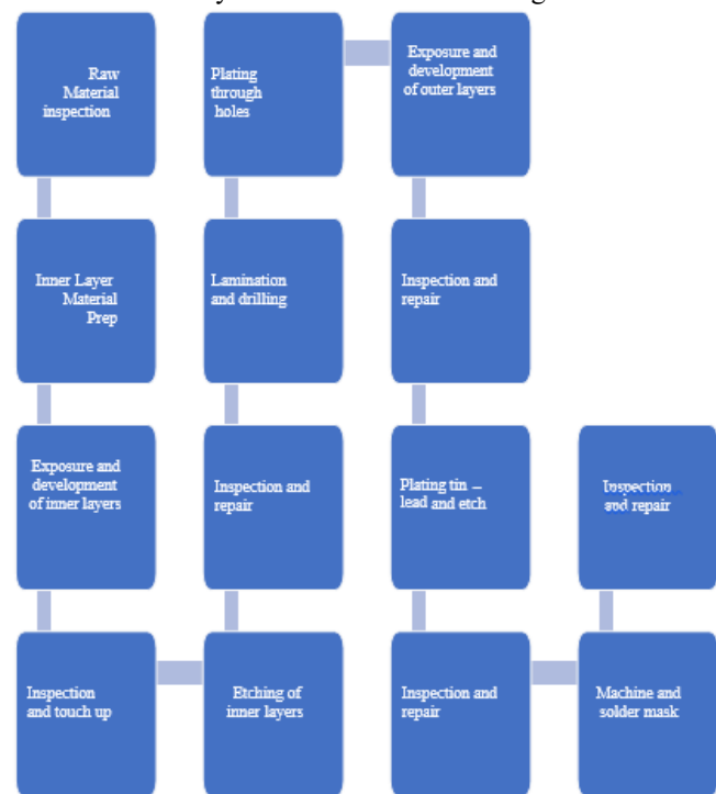
Fig.1: Printed Circuit Board Manufacturing Flow Diagram
