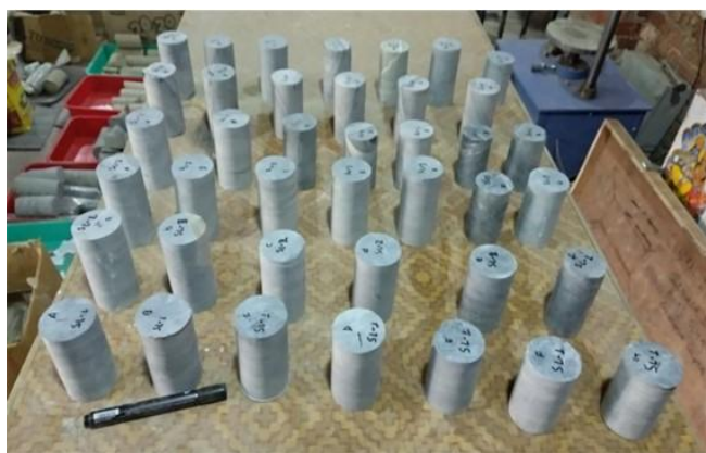
[Photograph 1: Sample Preparation of Selected Slate Specimens for the UCS Tests]
