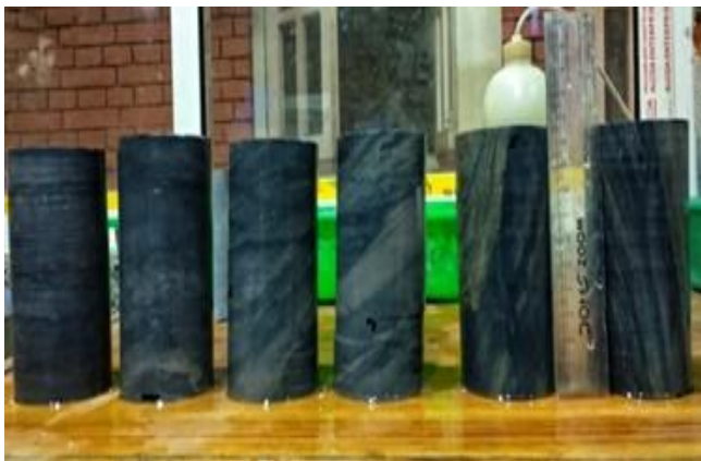
[Photograph 2: Core Samples Prepared at Lab on Different Foliation Angle]
