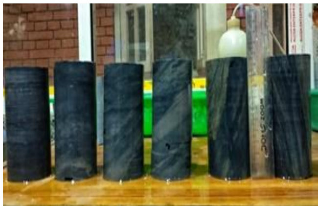
[Photograph 2: Core Samples Prepared at Lab on Different Foliation Angle]
