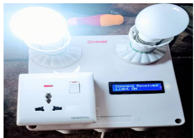
[Fig.8: Picture of the Implemented System for Light Control]
