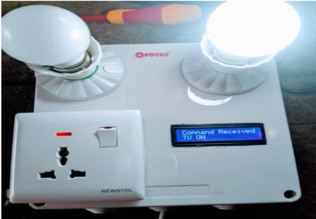
[Fig.9: Picture of the Implemented System for Television (TV) Control]
