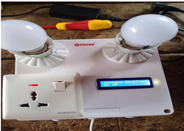
[Fig.10: Picture of the Implemented System for Air Conditioner Control]
