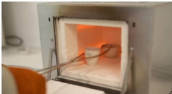
[Fig.2: Muffle Furnace for Determining Loss on Ignition]
