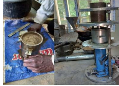
[Fig.3: Compaction Device]
