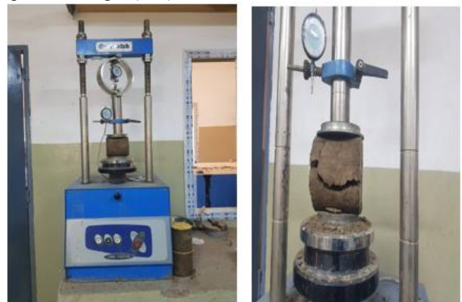
[Fig.6: a) CBR Press, b) Bending Device]
