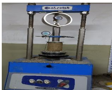
[Fig.5: a) CBR Press, b) Compression Device, Tensile Strength (Brazilian Test)]
