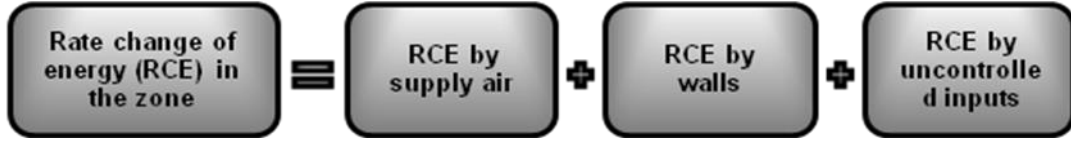
Figure 1. View of energy and mass balance equation that used for the zone modeling
