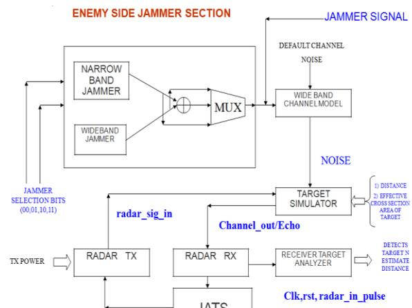
Fig 1: Frequency Agile Radar Blocks Diagram
