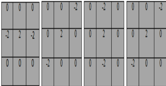
Fig. 3. Four edge thinning masks ( 0^\circ, 45^\circ, 90^\circ, 135^\circ )
