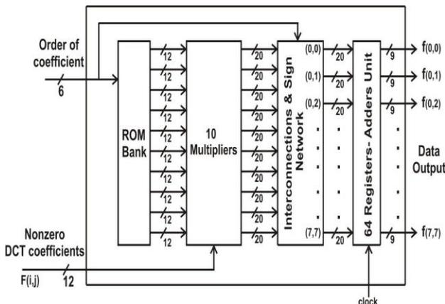
Fig. 3. 8x8 2D IDCT architecture
