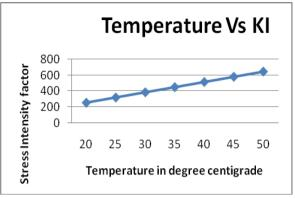
From the above graph it is observed that the temeprature is linear with the stress intensity factor.
