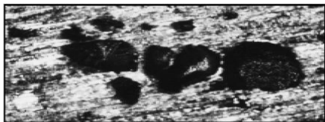
Figure 2: Gas porosity with medium (top figure) and large sized pores (bottom figure).
