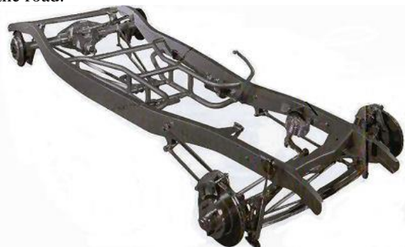
Fig2. Chassis of a sports car
