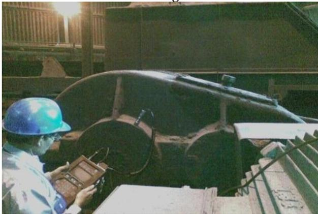
**Fig .5 Taking readings of output gear shaf**
