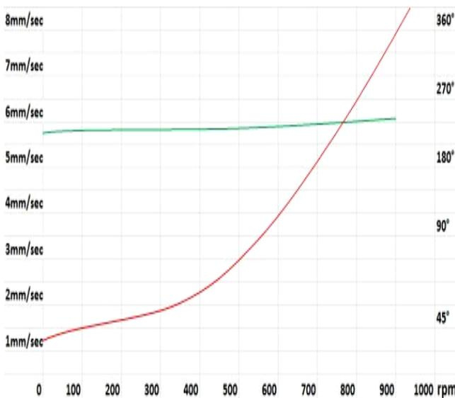
**Fig.7 BODO PLOT:** This graph gives the phase and amplitude difference at a time in coast down test
