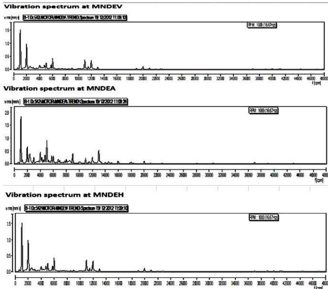
**Fig 8. Spectrums of the motor in vertical, horizontal and axial directions are taken with vibxpert. The spectrum is in RMS (mm/sec) vs. frequency (cpm)**
