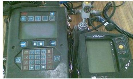
Fig.3 CSI and VIBXPERT, vibration analyzers
