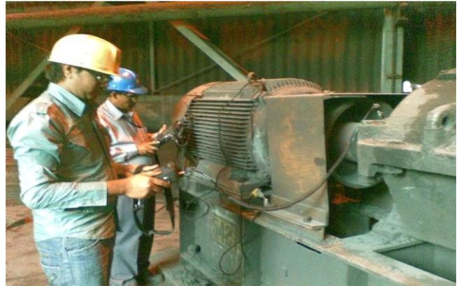
**Fig6. Taking vibration readings at MDE and MNDE**
