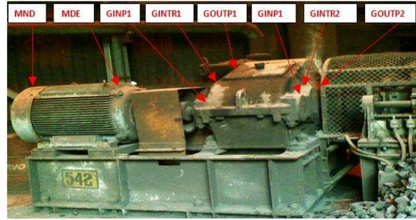
FIG2: monitoring points of motor and gear box.
