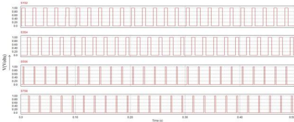
Fig. 14. Switching Pulses for Inverter
