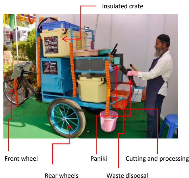
Fig.2. View of the innovative mobile fish vending unit for retail fish marketing
