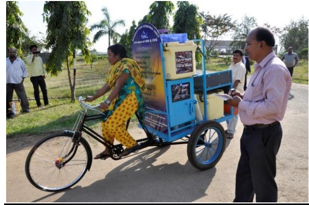
Fig.3. Ergonomical evaluation of trolley rickshaw by female operator
