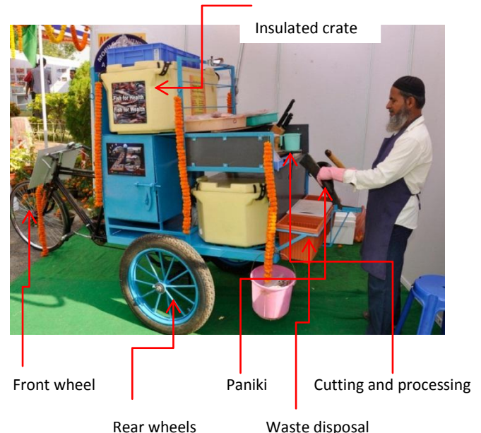
Fig.2. View of the innovative mobile fish vending unit for retail fish marketing
