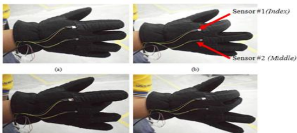
Fig 5: The example of GloveMAP Bending activities (a) straighten fingers (b) bending of index finger (c) bending of middle finger (d) bending of both fingers [27]
