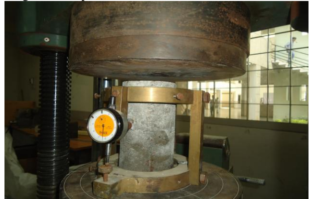
Fig:2 Setup of Compression Test
