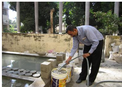
Fig 2: Setup of hot water curing
